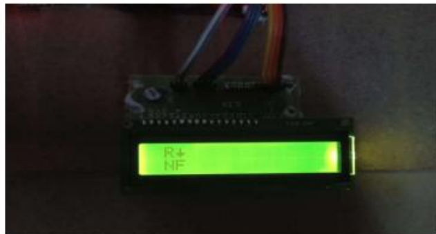
Fig. 7 No Fault Indication
