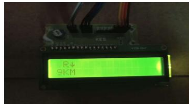
Fig. 8 Fault Indication at 9Km distance
